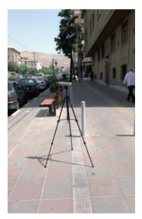
Figure 2. Placement of sound level meter on sidewalk to measure traffic noise
