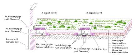
Figure 3. Schematic of the planting roof structure
