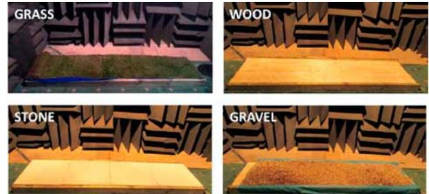
Fig. 2. The wooden platform used for the experiment, covered in turn with the four selected materials
