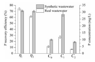
Fig. 4. P concentrations in the influent and effluent of IC column and its recovery efficiencies from synthetic and real wastewater
