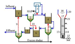
Fig. 1. Schematic diagram of the BNR-IC process.1– anaerobic tank; 2– settling tank; 3– IC column; 4– nitrification tank; 5– settling tank; 6– anoxic tank; 7– post-aeration tank; 8– settling tank; 9– sludge return; 10– sludge bypass return; 11– sludge return; 12– later flow; 13– influent of P-rich solution; 14– feeding CaCl2 solution; 15– aeration; 16– IC reaction zone; 17– buffer zone; 18– settling zone; 19– sample point; 20– effluent
