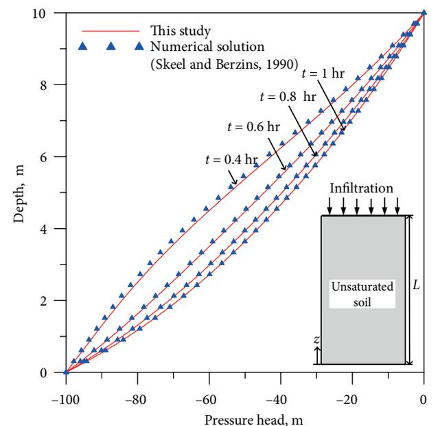
Fig. 6. Result comparison of verification example 2 with the numerical solution
