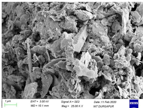
Figure 11. SEM micrograph of additive stabilized soil
