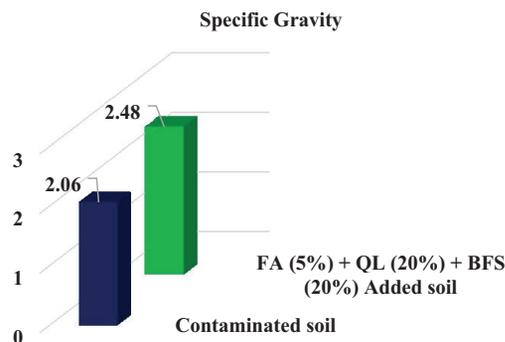
Figure 4. Comparison of Specific Gravity values of contaminated and additives stabilized soil
