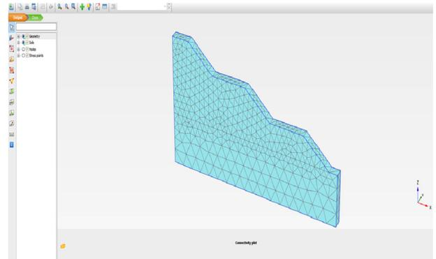
Figure 7. PLAXIS<sup>TM</sup> 3D model generated mesh diagram of the embankment (1 V: 1.5 H)
