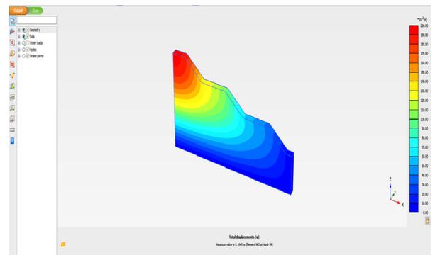
Figure 8. The vertical displacement of the embankment founded on contaminated soil (drained condition)
