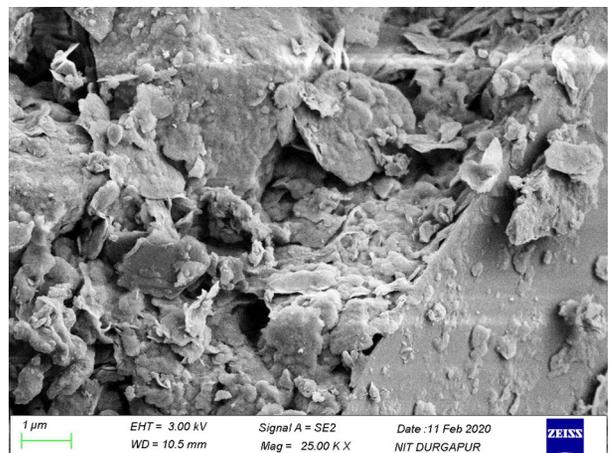
Figure 10. SEM micrograph of heavy metal contaminated soil
