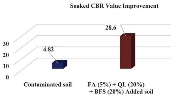
Figure 6. Comparison of soaked CBR values of contaminated and additives stabilized soil
