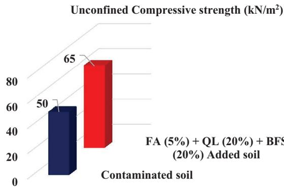
Figure 5. Comparison of UCS values of contaminated and additives stabilized soil
