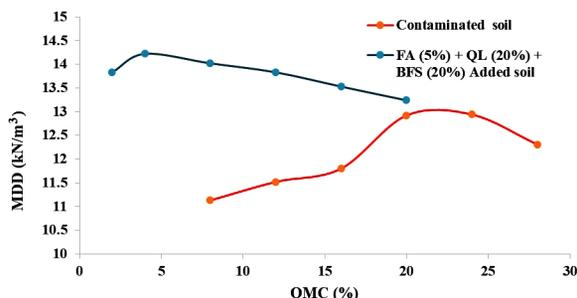
Figure 3. Comparison of compaction characteristics of contaminated and additives stabilized soil
