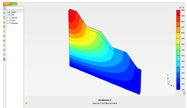
Figure 9. The vertical displacement of the embankment founded on stabilized soil (drained condition)
