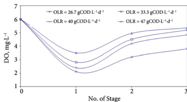
Fig. 3. DO concentration profiles in different stages of RBC with various OLR
