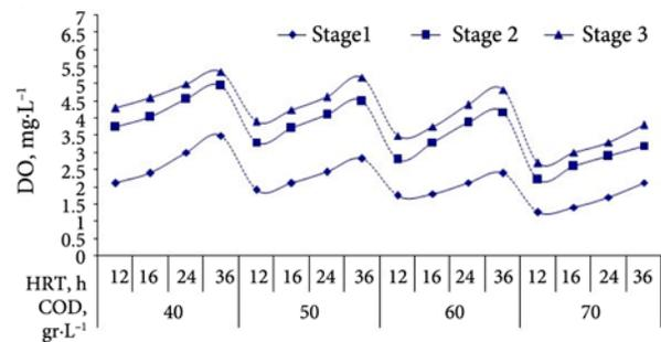
Fig. 2. DO level with respect to HRT and COD in different stages
