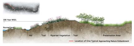
Figure 3. Cross-section of one typical approaching nature embankment
