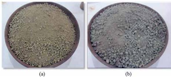
Fig. 2. Photographs (a) Soil sample from D.G. Khan (CL), (b) Soil sample from Nandipur (CH)
