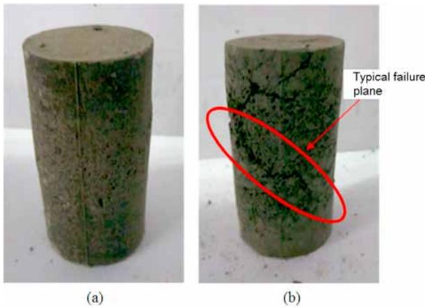
Fig. 14. Typical unconfined compression test specimens (a) before test (b) after test
