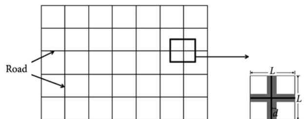
Fig. 6. Square grid layout of road network. Within each unit area, the edge effect of roads is in gray strips
