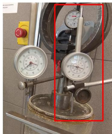
Figure 4. The location of the annular surcharge ring displacement sensor in the CBR loading press
