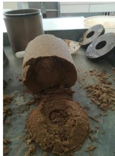
Figure 3. The view of the soil sample after the CBR test
