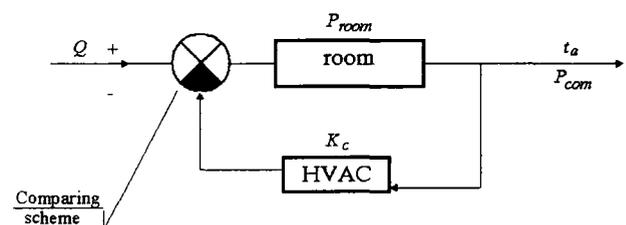
Fig 1. The automatic control circuit of the indoor microclimate
