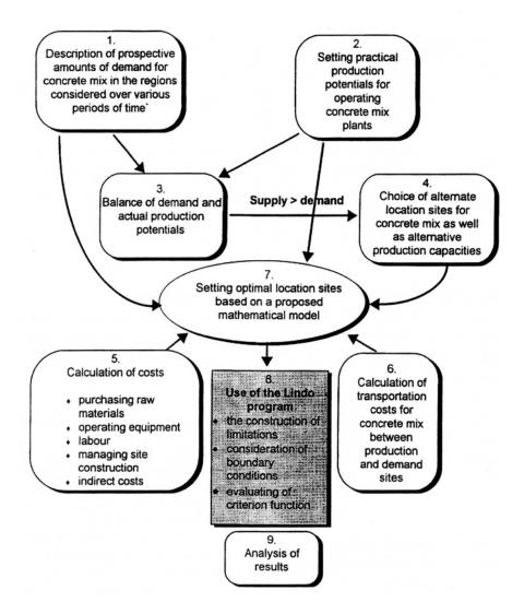
Fig 5. Diagram of functions necessary to obtain optimal location sites
