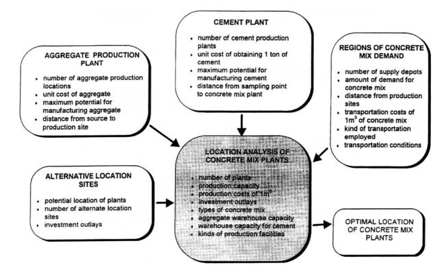
Fig 4. Location factors within individual elements of a production process
