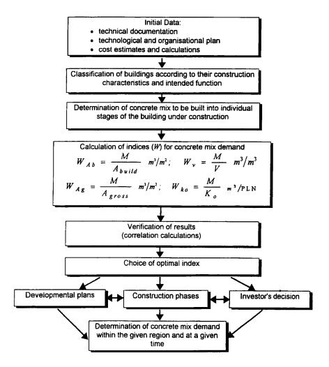
Fig 1. Algorithm for obtaining the given amount of concrete mix demanded: M - amount of concrete mix  $[m^3]$ ;  $A_{build}$  - area of building  $[m^2]$ ;  $A_{gross}$  - gross area  $[m^2]$ ; V - volume of building  $[m^3]$ ;  $K_0$  - estimated value [PLN]
