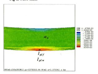
Fig 9. Distribution of plastic deformation in the bisteel beam
