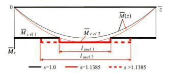
Fig 6. Distribution of elastic capacity moments
