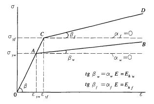
Fig 2. Stress-strain diagram
