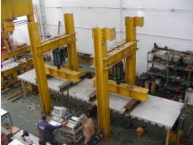
Fig 6. Testing in laboratory of CTU in Prague: General set-up (left), slip measurement (right)
