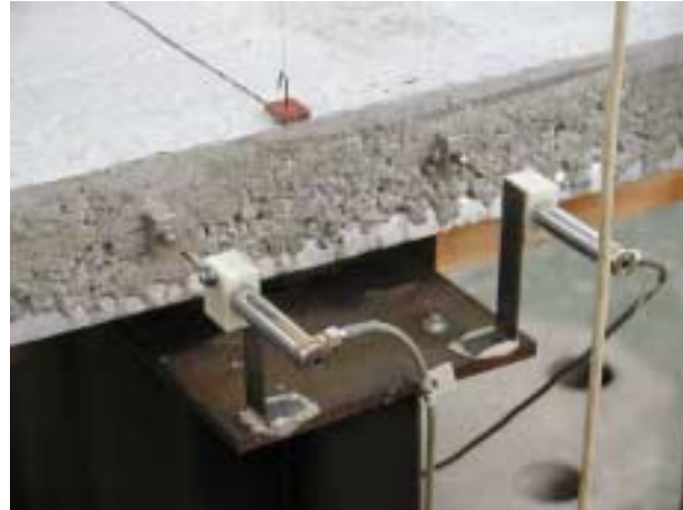
Fig 6. Testing in laboratory of CTU in Prague: General set-up (left), slip measurement (right)
