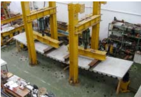
Fig 8. Girder in test EX1 after collapse
