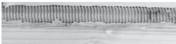
Fig 3. Adhesion of implant thread to timber when angle of screw \alpha = 0^\circ
