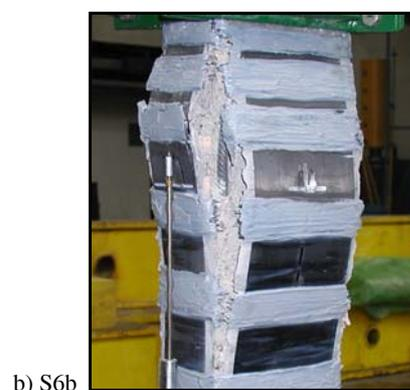
Fig 7. Damaged elements from series “a”
