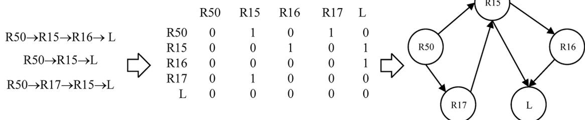
Figure 2. Formative process of a part of cost overrun risk propagation network (CORPN)
