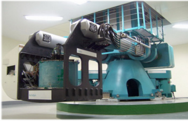
Fig. 1. Centrifugal model test apparatus (KOCED Geocentrifuge center at KAIST)
