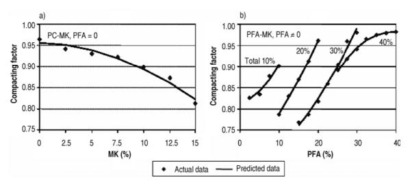
Fig. 2. Comparison and prediction of compacting factor with statistical models
