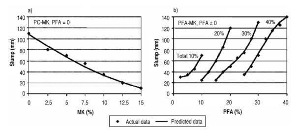
Fig. 1. Comparison and prediction of slump with statistical models
