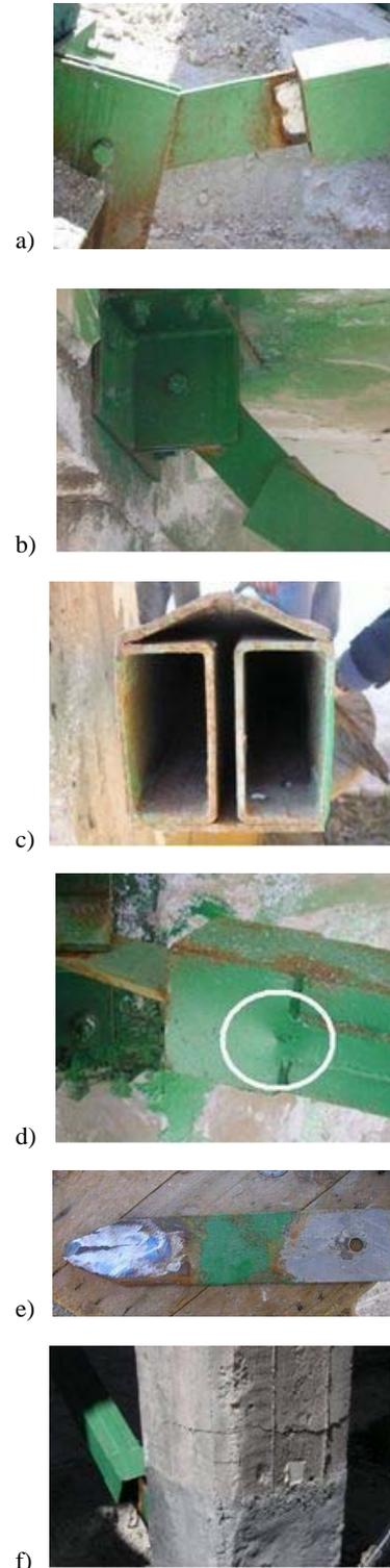
**Fig. 16.** Test No. 1 on BRBs: damage pattern
