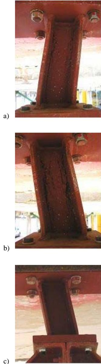
Fig. 12. Test No. 3 on EBs: ductile shear hinging of links
