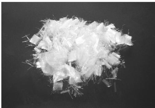
Fig. 1. Polypropylene fibers used
