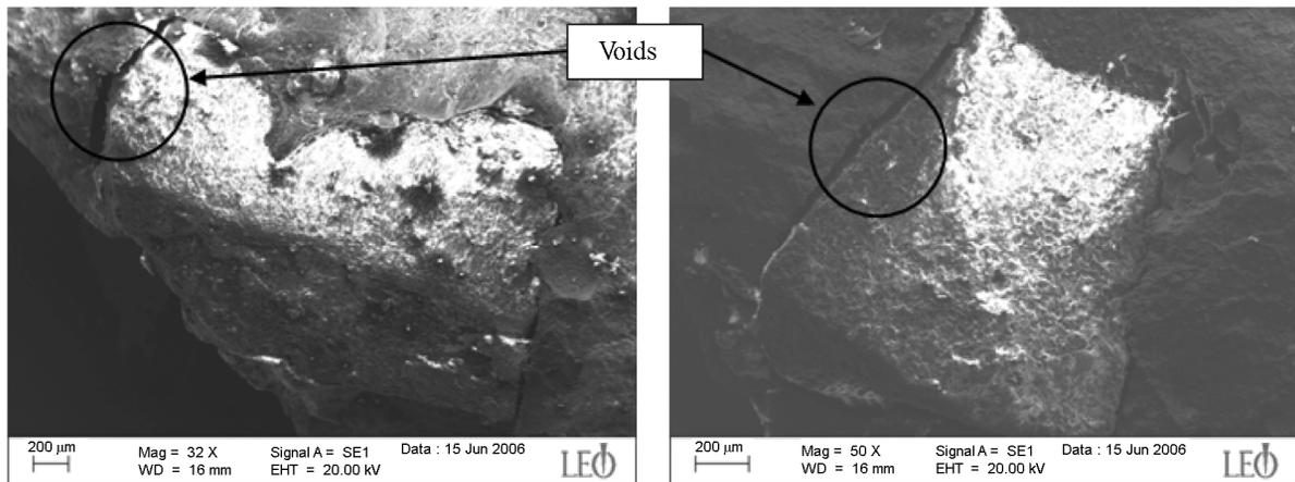
Fig. 3. SEM image of the concrete including APS
