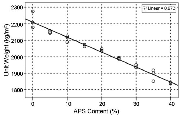
Fig. 2. Relationship between unit weight and APS content
