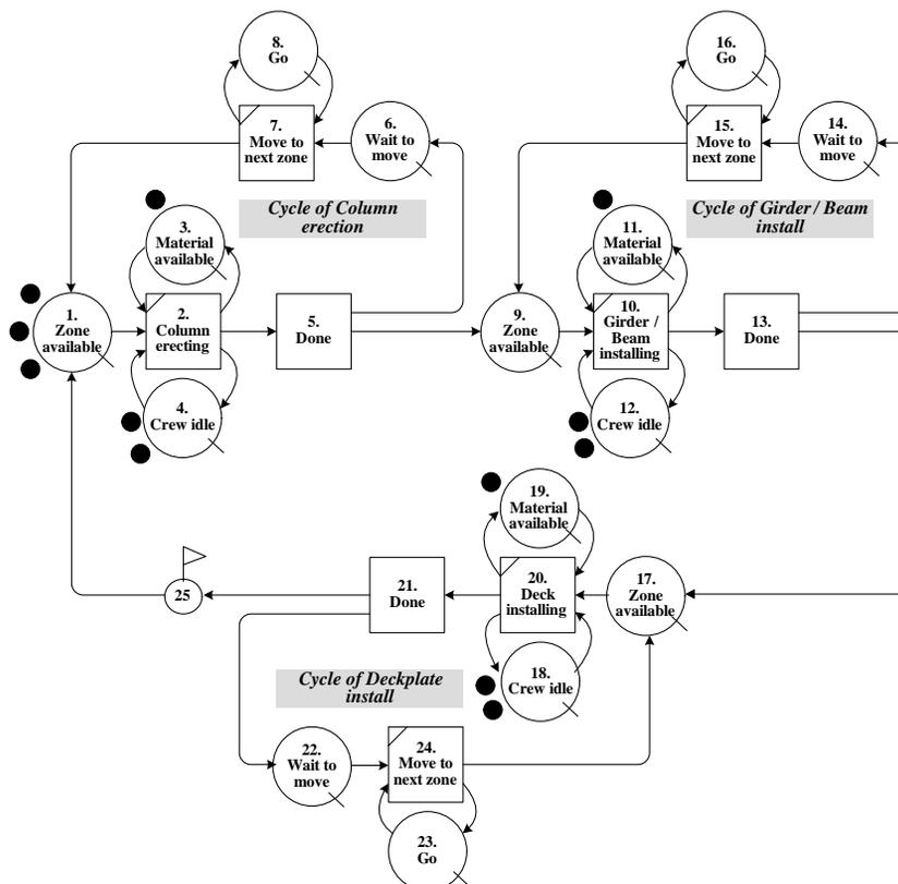
Fig. 4. SCHEME for steel structure construction
