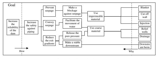
Fig. 5. FAST diagram for the dam
