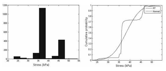
Fig. 6. Histogram and CDF of pore pressure in horizontal drain level
