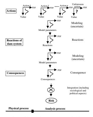
Fig. 1. Risk analysis processes for a typical dam
