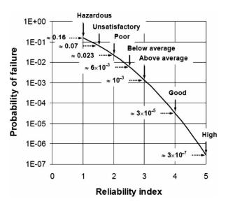
Fig. 2. Assessment of dam safety levels with the reliability index
