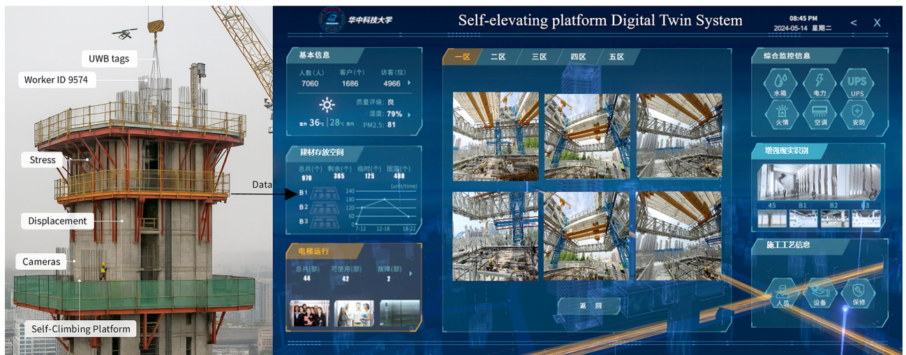
Figure 20. Architecture of the digital twin and multi-source integration for self-climbing platform operations
