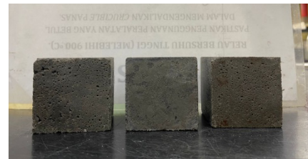
Figure 13. Appearance of fresh mortar cubes
