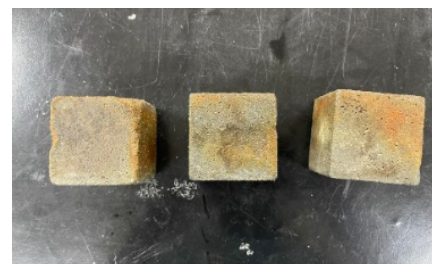
Figure 13. Appearance of fresh mortar cubes
