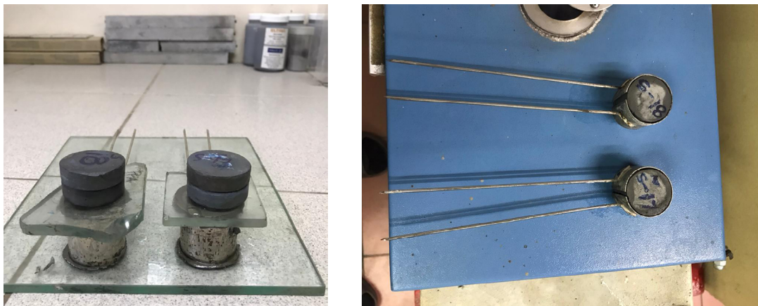
Figure 7. Soundness test samples
