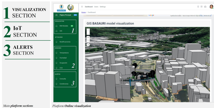
Figure 6. Main blocks of the platform
