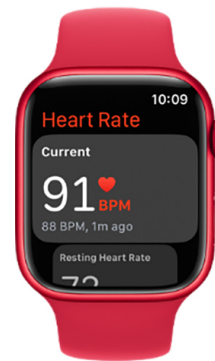
Figure 2. Sample of the Apple Watch Series 4 1 , which was used to capture the heart rate of construction workers
