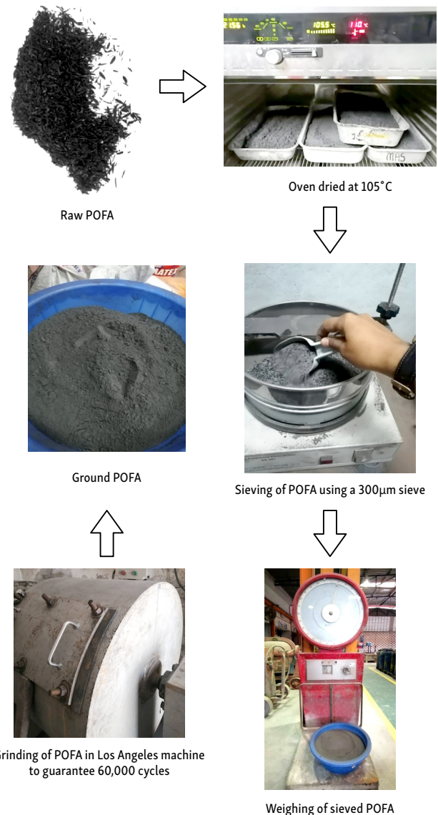
Figure 2. Procedure of preparing finer POFA
