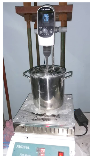
Figure 3. Extraction of IHS using hydrothermal method
