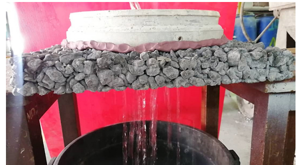
Figure 12. Infiltration test of GPC
