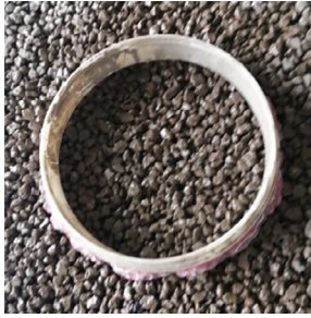
Figure 7. Infiltration test on GPC paver
