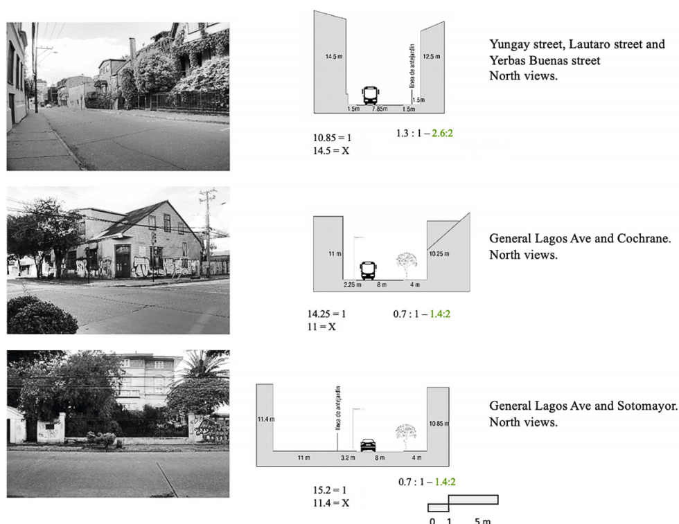
Figure 10. Radio study of height vs. width of street, Zone 1
