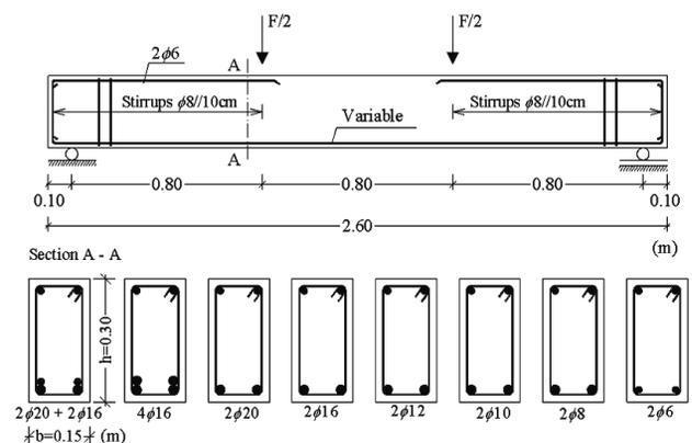
Fig. 1. Geometry and details of test beams (Bernardo *et al.* 2014)
