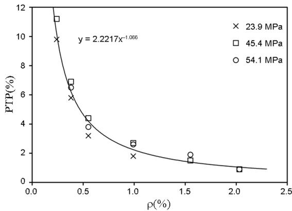
Fig. 9. Influence of reinforcement ratio on the PTP
