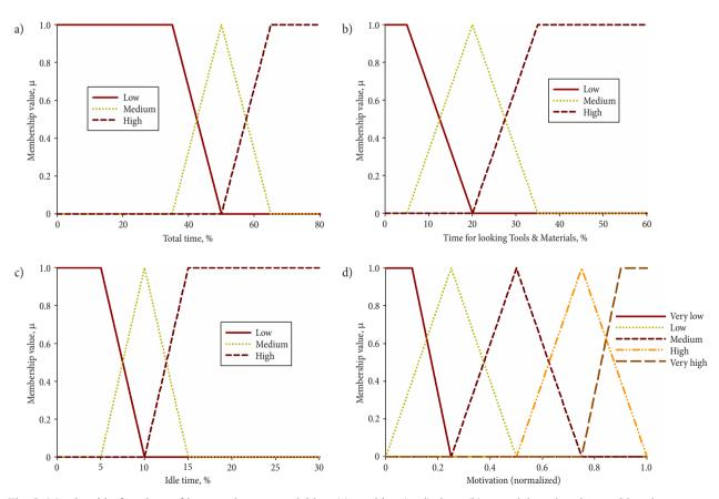
Fig. 2. Membership functions of input and output variables: (a) working (tool) time, (b) materials and tools searching time, (c) idle time, and (d) motivation
