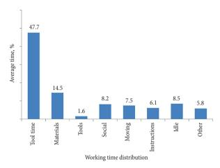
Fig. 1. Working time distribution of the 38 construction workers
