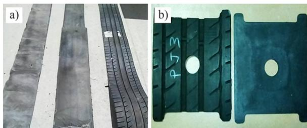
Fig. 1. a) Tire layers: inner (left), middle (center) and outer (right). b) Rail pad made of deconstructed EOL-tires (left); commercial rail pad made of crumb rubber particles (right)
