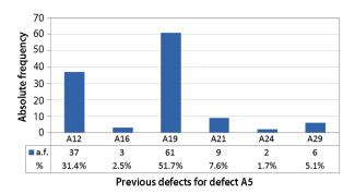
Fig. 18. Absolute frequency (a.f.) and percentage of previous defects for defect A5 - linear cracking
