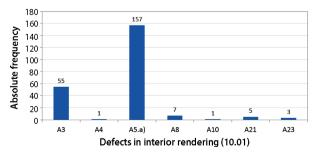
Fig. 23. Absolute frequency of defects in interior rendering (10.01)
