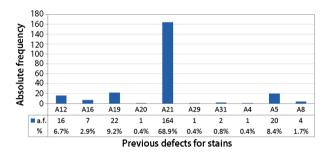
Fig. 27. Absolute frequency (a.f.) and percentage of previous defects for stains (A3) in the case studies
