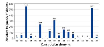
Fig. 11. Absolute frequency of defects according to the construction elements
