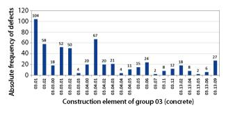
Fig. 10. Absolute frequency of defects according to the specific construction elements belonging to group 03 - concrete elements
