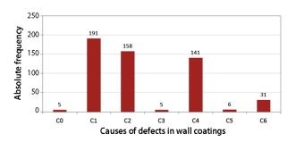
Fig. 25. Absolute frequency of the general groups of causes in wall coatings (10)
