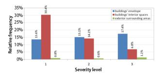
Fig. 9. Percentage of defects diagnosed, according to their level of severity, in the buildings' envelope, in interior areas and in external surrounding areas
