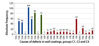
Fig. 26. Absolute frequency of the specific causes of anomalies in wall coatings (10) belonging to general groups C1, C2 and C4
