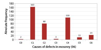
Fig. 16. Absolute frequency of the general groups of causes in masonry (06)
