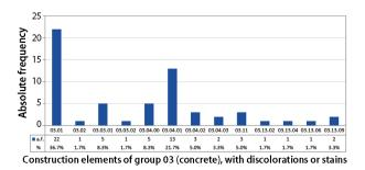
Fig. 29. Absolute frequency (a.f.) and percentage of specific construction elements belonging to group 03 – concrete elements with discolorations or stains (A3)
