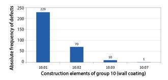
Fig. 22. Absolute frequency of defects according to the specific construction elements belonging to group 10 - wall coatings
