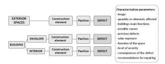
Fig. 5. Organogram of the parameters included in the characterization of the school buildings section
