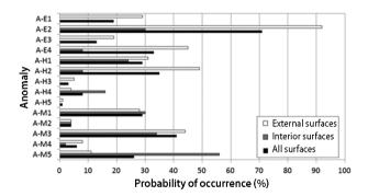
Fig. 24. Probability of finding each anomaly in one wall considering external surfaces, interior surfaces and all surfaces (adapted from Sá *et al.* 2015)
