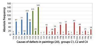
Fig. 21. Absolute frequency of the specific causes of anomalies in paintings (20) belonging to general groups C2 C1, and C4
