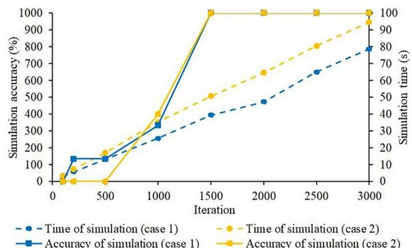
Figure 5. Simulation iteration selection for PSO-based optimization
