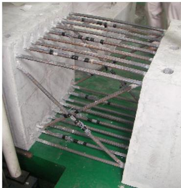
Fig. 6. Strain gauges
