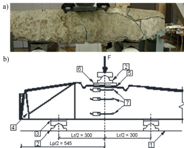
Fig. 4. Arrangement of strain measurement devices: a) testing view with DEMEC gauges; b) testing scheme with LVDT gauges. 1 – rigid support; 2 – hinge support; 3 – elastic pad; 4 – prestressed concrete monoblock sleeper; 5 – standard rail pad; 6 – inclined plate
