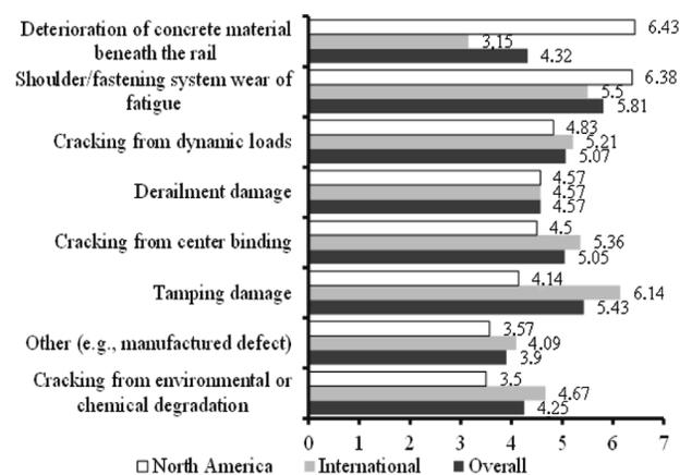
Fig. 1. Main failure causes of concrete sleeper (Dyk *et al.* 2012)
