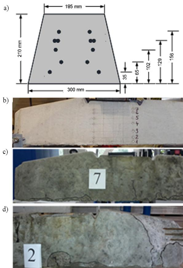
Fig. 2. Prestressed concrete sleepers: a) cross-section; b) new sleeper; c), d) used sleeper
