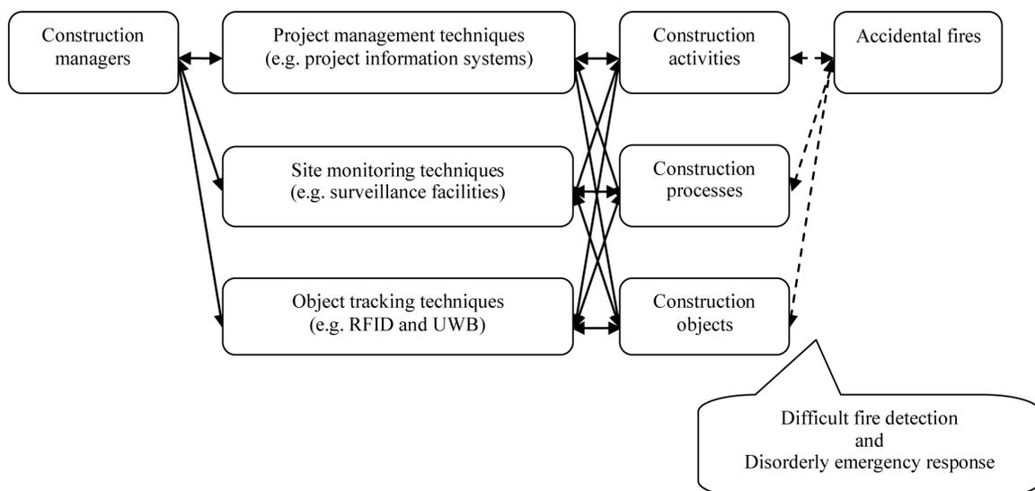
Fig. 1. Using information techniques for construction site safety management
