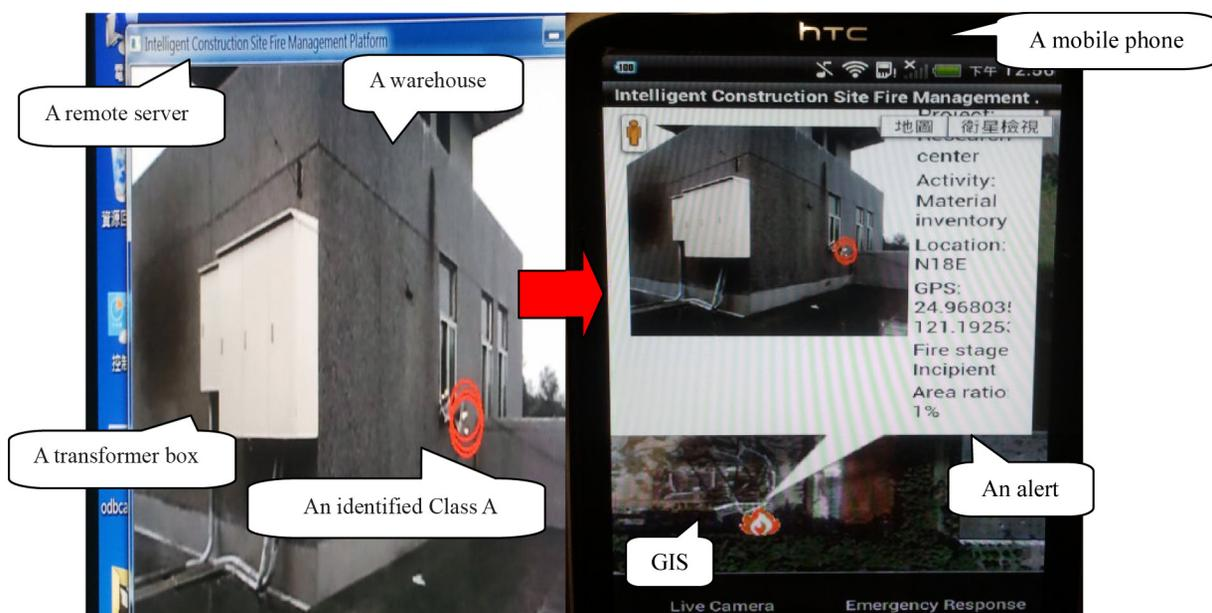
Fig. 4. Image-recognition-based mechanism for a Class A fire
