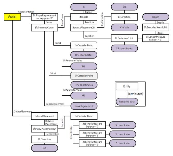
Fig. 2. Data extraction path in IFC
