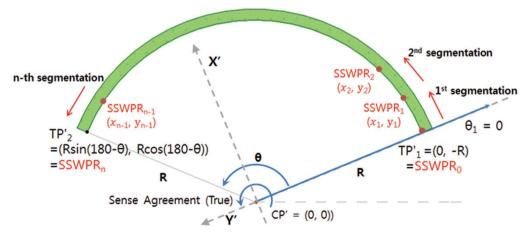
Fig. 5. Concept of rotated  $SSWPR_n$  based on CP'
