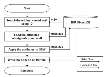
Fig. 10. Process of generating INP file
