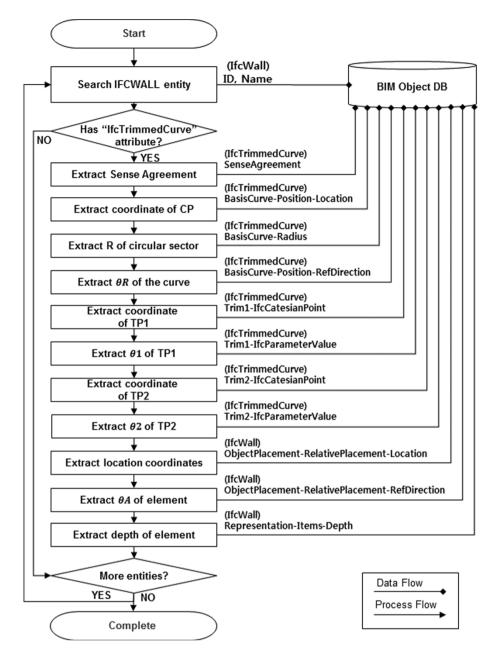
Fig. 4. Process to extract data from IFC
