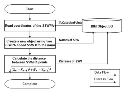
Fig. 8. Process to create SSW<sub>n</sub>
