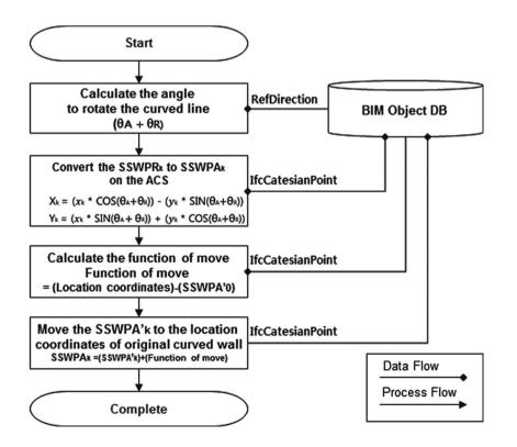
Fig. 7. Process of **SSWPA**<sub>n</sub>
