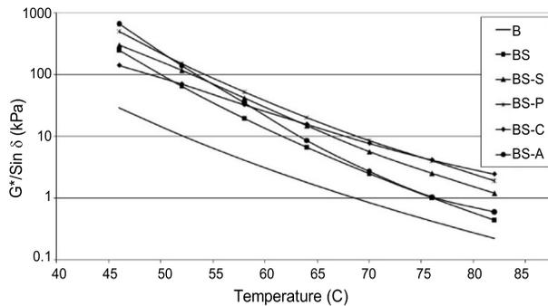
Fig. 8.  $G^*/\text{Sin } \delta$  for bitumen binder aged with RTFO at 1.59 Hz
