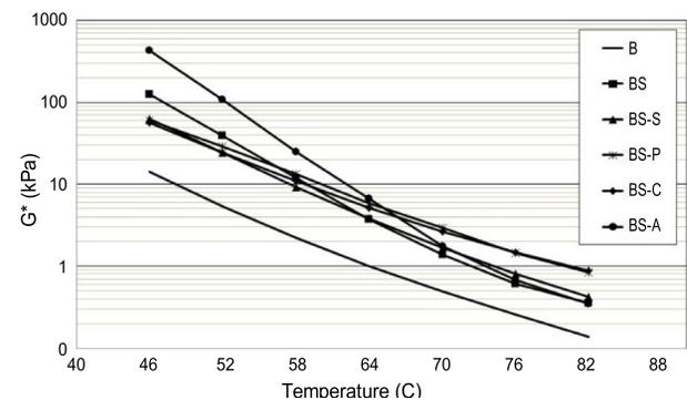
Fig. 6. The parameter  $G^*$  versus temperature for unaged base and modified bitumen
