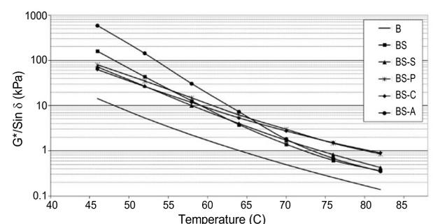
Fig. 7.  $G^*/\sin \delta$  for unaged bitumen binder at 1.59 Hz
