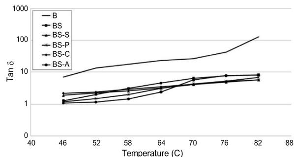
Fig. 9. Plot of tan  $\delta$  against temperature for study binders at constant frequency of 1.59 Hz
