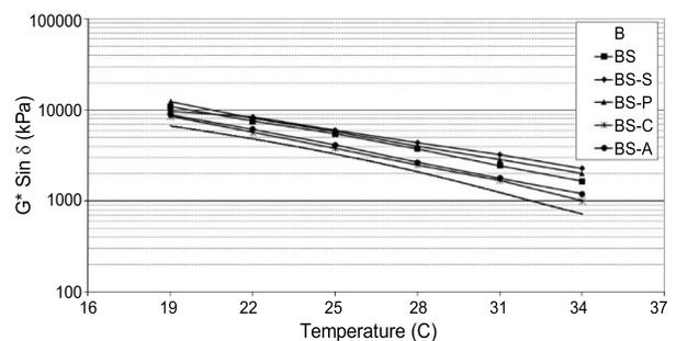
Fig. 10. Plot of  $G^*.\text{Sin } \delta$  for binders aged with PAV
