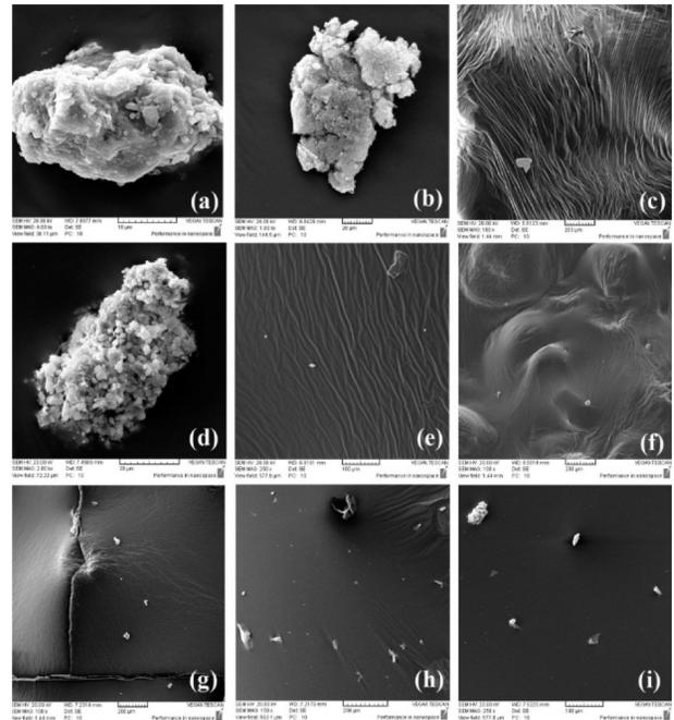
Fig. 4. SEM images of various additive types of the study: a) Sasobit; b) Crumb rubber; c) Polyphosphoric acid; d) SBS; e) Anti-stripping agent; f) Sasobit - CR distribution; g) Sasobit - PPA distribution; h) Sasobit - Anti-stripping agent distribution; i) Sasobit - SBS distribution
