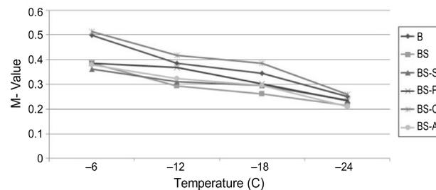
Fig. 11. M-value of binders at low temperature range
