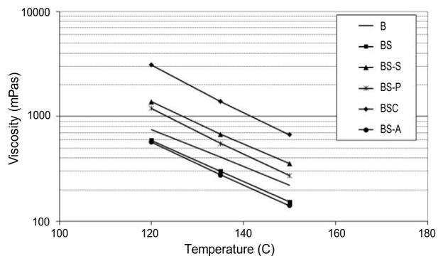
Fig. 5. Dynamic viscosity curves of modified bitumen
