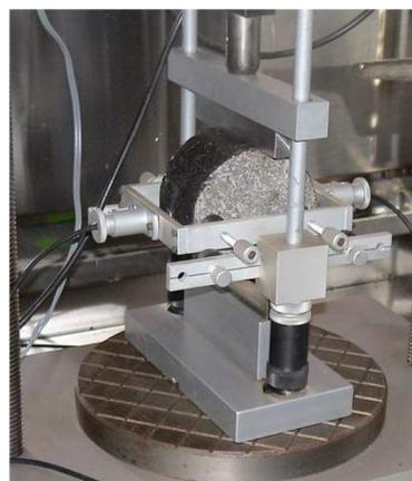
Fig. 2. The indirect tensile stiffness modulus test apparatus
