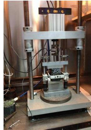
Fig. 3. The indirect tensile fatigue test apparatus
