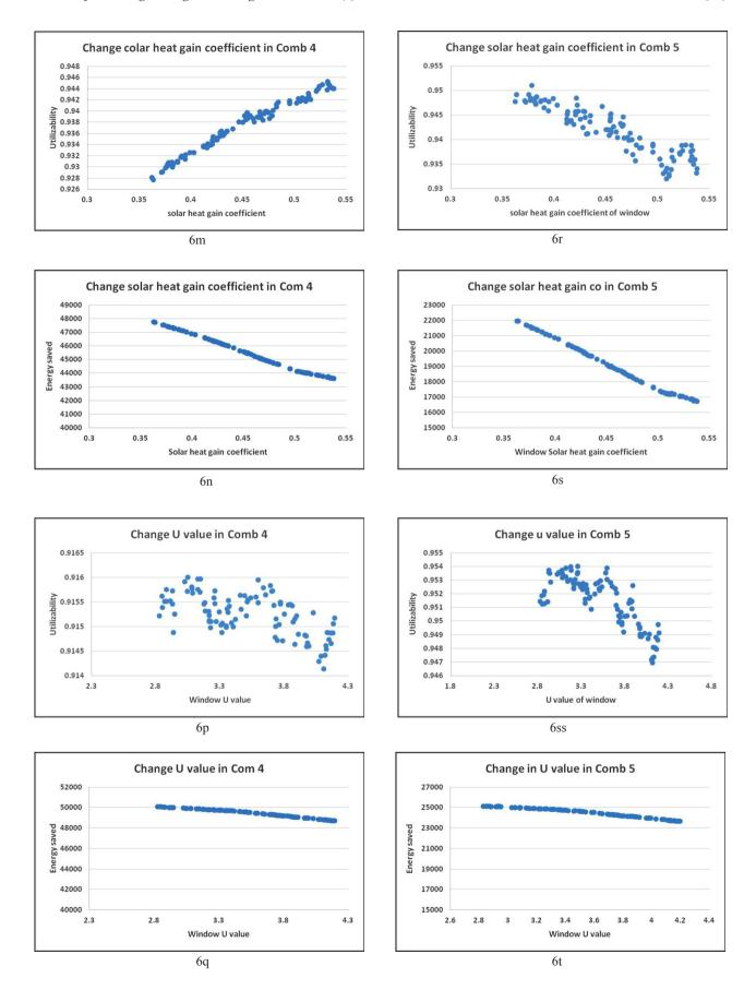
Fig. 6. Change of utilizability and energy saving with varying parameter (m-t)
