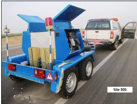
Fig. 3. FWD testing and depth temperature measurements of asphalt layers on a pavement site
