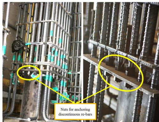
Fig. 3(c). Discontinuous re-bars connected to steel plates by bolts (Specimen #3; 12 re-bars cut off)
