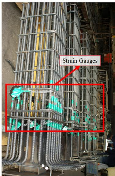
Fig. 5. Strain gauges of re-bars
