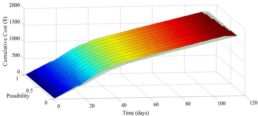
Fig. 14. Project S-Surface without task overlaps
