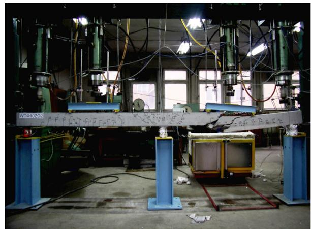
Fig. 12. The destroyed beam no. 1
