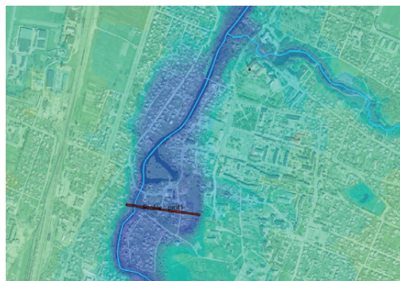
Fig. 5. Overlay of modeled water surface and area topography on the aerial photograph of the Akmena-Danė river basin area in the central part of Kretinga Town (grid 5 m). Potential flood risk zones are not shadowed
