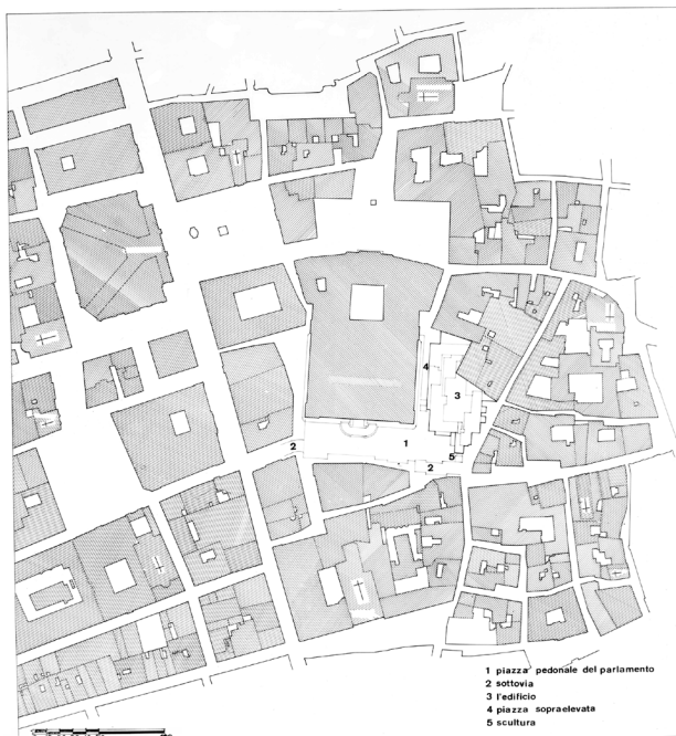
Figure 3. Site plan showing Basile's cubical addition in the medieval fabric of Rome. The upper portion of the building with a curvilinear facade is 17th century Lorenzo Bernini's palace commissioned by Pope Innocent X, later adopted by Carlo Fontana. Number 1 indicates the location of Piazza del Parlamento (source: IUAV Archivio Progetti, 1967)
