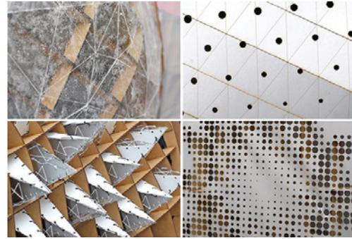
Figure 7. Details revealing different digital strategies for the solutions of the skin that cover shared curvature of the whole installation. From top left: triangulated transparent acrylic covered with silicone, laser perforated and engraved white cardboard, surface faces offset and extruded to acrylic pyramids that are bound together with a tread, laser perforated metallic-coated paper
